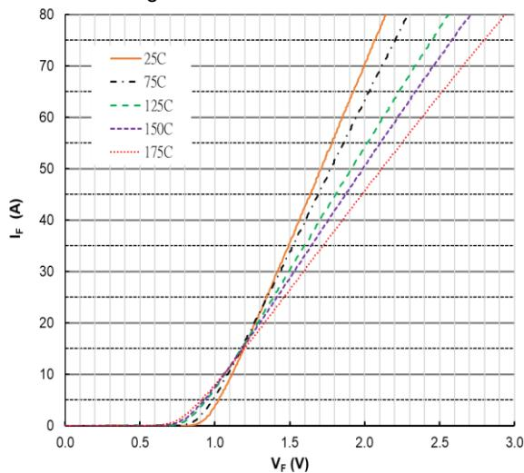
Figure 2. Forward Characteristics
